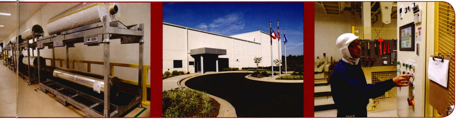
Above, from left to right: 1: Toppan's slitter machine, which cuts the finished film to the length and width specified by the client; 2-3: Toppan employees working with the film on the slitter; 4: rolls of raw film waiting to begin the coating and vacuum metallization process; 5: exterior of Toppan's new facility in Griffin, Ga.; 6: Kohei Suenaga monitoring conditions on the Coating machine.
